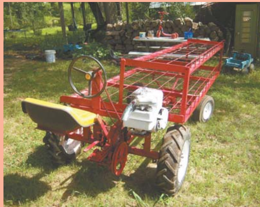
Low-profile garden cart measures 9 ft. long and has a 7-ft. long, 2-level table on front that holds up to 27 flats.
