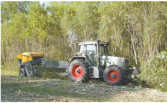
Forest undergrowth is reduced to small pieces after being cut and mulched by the BioBaler.
