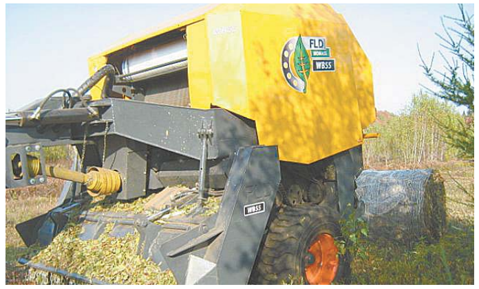
Baler has a 48-tooth rotor that chops a 7 1/2-ft. wide swath through heavy brush.
