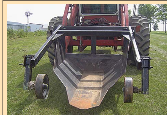
Loader can quickly be set up to tow behind a pickup or semi trailer, allowing it to be hauled down the road at highway speeds. It’s powerful enough to carry 3 big bales.
