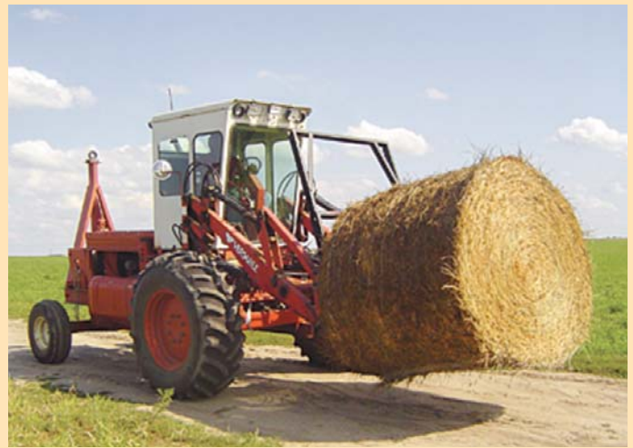
Dan Crick, Menno, S. Dak., rebuilt a 1976 IH 715 combine, and fitted it with a loader off a Versatile 256 bi-directional tractor.
