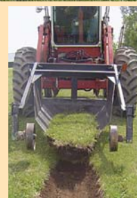
Ditch digging spade is 5 1/2 ft. long and has an 18-in. wide, rounded bottom. A pair of metal wheels keep the spade level and also control digging depth. “It works great for installing electric wire under the ground because I can dig sod out without going too deep,” says Crick.
