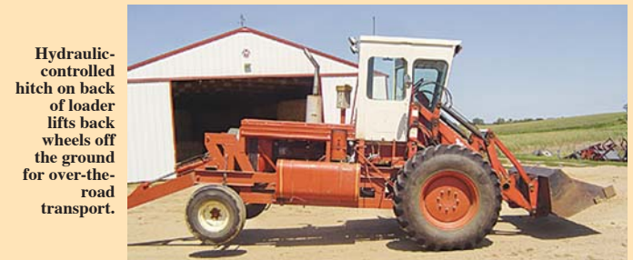
Dan Crick, Menno, S. Dak., rebuilt a 1976 IH 715 combine, and fitted it with a loader off a Versatile 256 bi-directional tractor.
