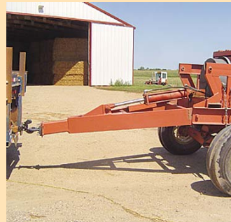
Loader can quickly be set up to tow behind a pickup or semi trailer, allowing it to be hauled down the road at highway speeds. It’s powerful enough to carry 3 big bales.
