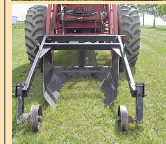
Rock picker bolts to loader bucket and is equipped with four steel spears made from 1 3/4-in. dia. spring steel. A metal lip on front of mounting frame serves as a “dam” to keep rocks from rolling back out of bucket. “It’s a simple idea but it’ll outpick any rock picker I know of,” says Crick. “There’s no need to dig out around the rock at all. I tilt the spears at an angle and slide them under the rock as I drive forward. Once the rock is on top of the spears, I bounce the bucket up and down a couple of times to shake off the dirt, and then tilt the bucket up until the rock rolls in.”
