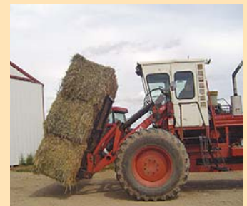
Loader can quickly be set up to tow behind a pickup or semi trailer, allowing it to be hauled down the road at highway speeds. It’s powerful enough to carry 3 big bales.
