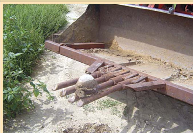
Rock picker bolts to loader bucket and is equipped with four steel spears made from 1 3/4-in. dia. spring steel. A metal lip on front of mounting frame serves as a “dam” to keep rocks from rolling back out of bucket. “It’s a simple idea but it’ll outpick any rock picker I know of,” says Crick. “There’s no need to dig out around the rock at all. I tilt the spears at an angle and slide them under the rock as I drive forward. Once the rock is on top of the spears, I bounce the bucket up and down a couple of times to shake off the dirt, and then tilt the bucket up until the rock rolls in.”
