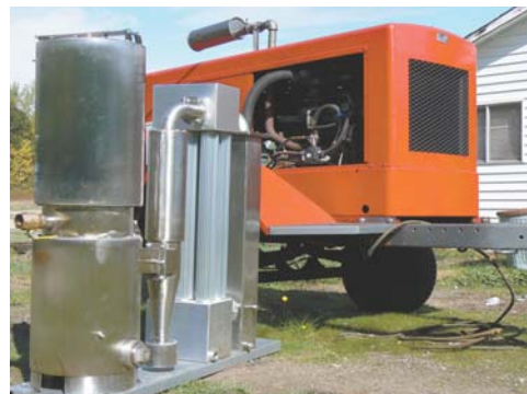
Ben Peterson uses his home-built gasifier to break wood down into gas that fuels a low-speed engine, which in turn charges a bank of batteries.
