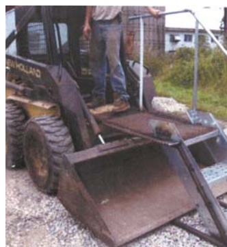
Simple platform (left) makes it easier to climb into a skid loader. Quick hitch (right) allows operator to hook up wagons without getting off tractor.
