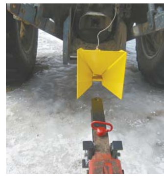
Simple platform (left) makes it easier to climb into a skid loader. Quick hitch (right) allows operator to hook up wagons without getting off tractor.
