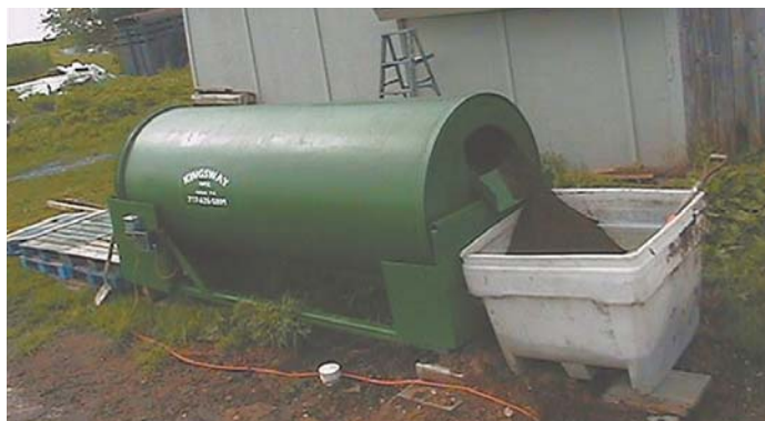
Kingsway composters range in size from 300 to 20,000 gal. The 1,000-gal. model shown above is the company's smallest continuous flow model.
