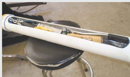
"Slide out" toolbox is designed to fit into the loader arms on Godbey's Deere skid loader. It consists of a length of 4-in. dia. pvc pipe with one side cut out.
