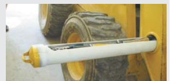
Toolbox fits in existing tube hole in skid loader's lift arms.
