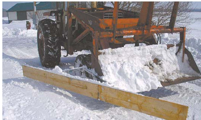
"Snow ridge remover" consists of a 12-ft. long, 2 by 12 wood board that bolts to the side of Pederson's loader bucket.
