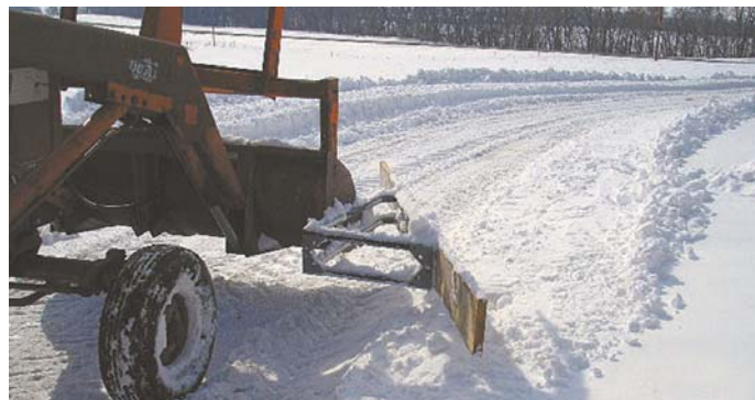
Board is bolted to a V-shaped metal frame, set at a 30-degree angle to bucket.
