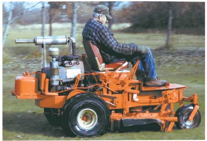
Mower is powered by swather's original 4-cyl., 28 hp Wisconsin engine and is equipped with a 60-in. Arts Way mower deck.
