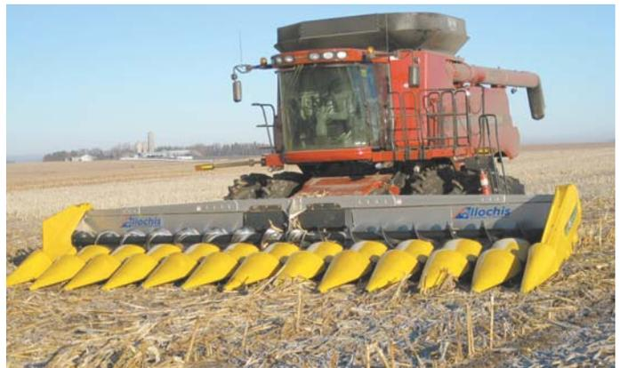
Low-profile Allochis corn header is available in either aluminum or steel. Features include hydraulic-operated stripper plates and clear plastic inspection windows in the shields.
