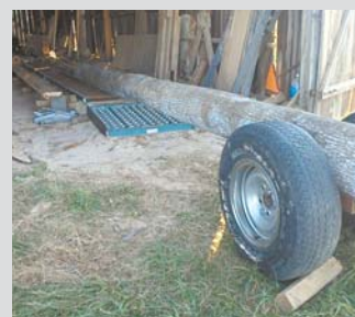
Home-built log caddy is used to move log forward and down the conveyor's length.
