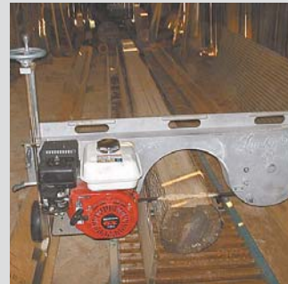
Lumber Smith Portable Sawmill weighs only 105 lbs., including the 5 1/2 hp Honda engine that drives it.
