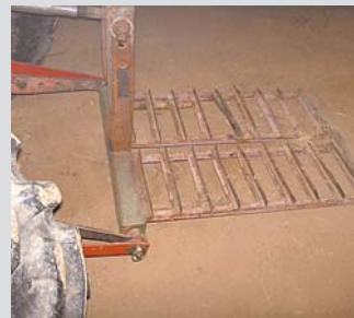
Bowman made this 3-pt. mounted carrier to carry larger logs to saw. Adjustable stops hold logs in place.
