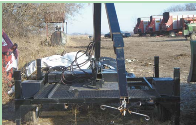
Lift mounts on trailer, making it easy to move where needed.
