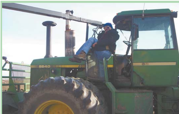
Hydraulic lift lets Duane Pung get up into a tractor. Canvas sling attaches to hooks on boom.
