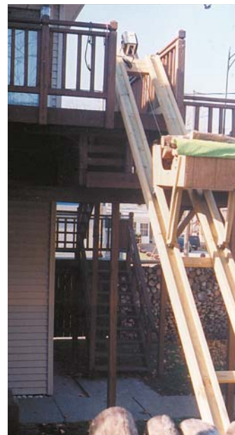
Winch-powered cart is used to haul firewood up to deck on second floor apartment. Winch at top of ramp is remote controlled.
