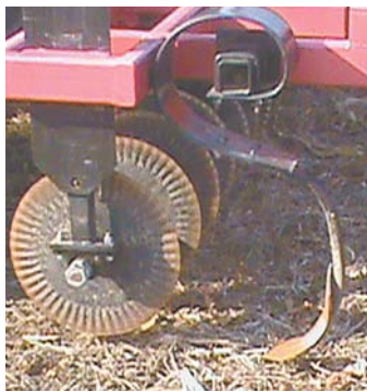
"My 12-ft. Chisel Ripper leaves the soil open for corn roots to go deep into the ground," says inventor Jeff Sberna.
