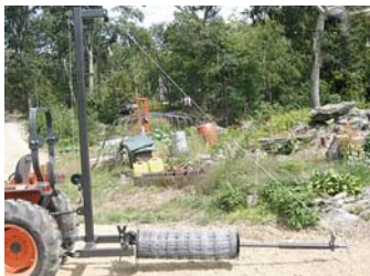
Spindle drops down to load roll of wire.
