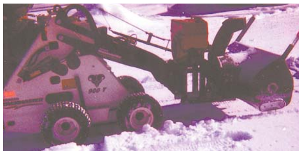
A 48-in., 2-stage snowblower was adapted to fit a Ramrod 900 mini skid loader.
