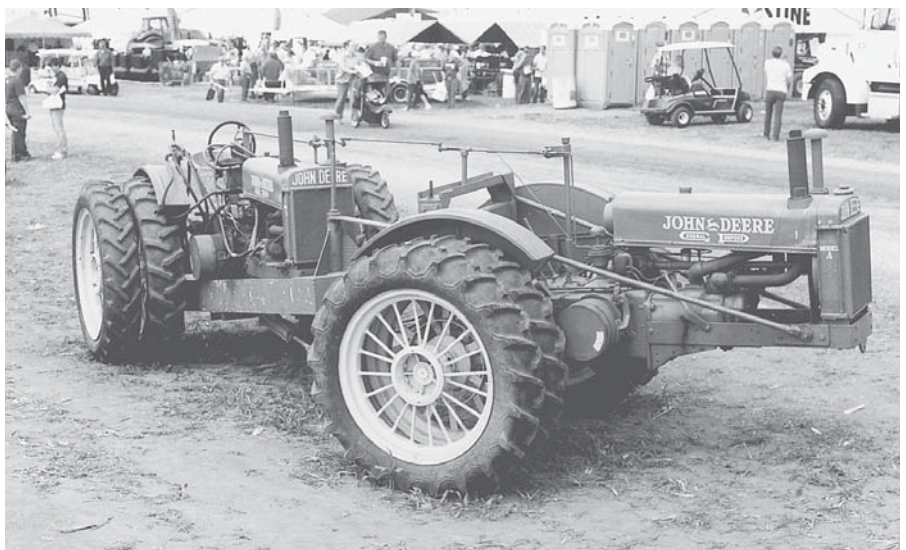
Tandem tractor was built from two Deere A's, both equipped with dual wheels.
