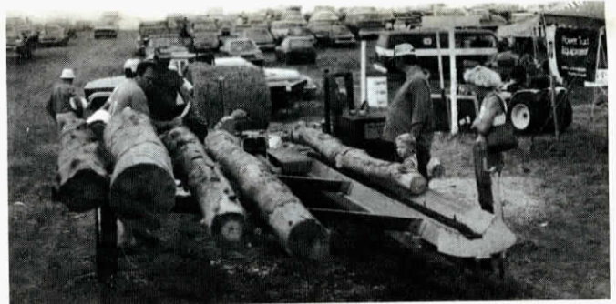
Once logs are loaded, machine automatically cuts and splits them into firewood.
