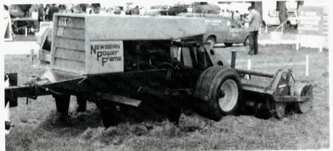
Newbern 122 hp. engine mounts above the chisel shanks and powers the rear roto-tiller.
