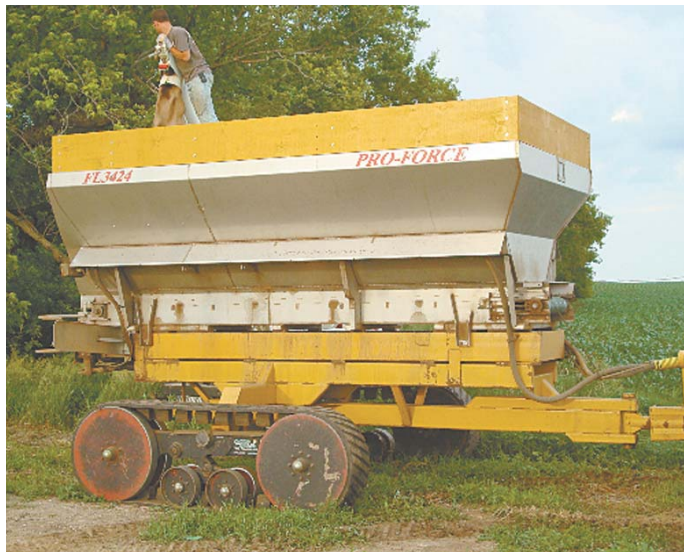
Dry fertilizer applicator rides on custom-made frame and tracks. Articulating hitch allows cart to follow in the tracks of the Mulvihills' Cat tractor as it turns.
