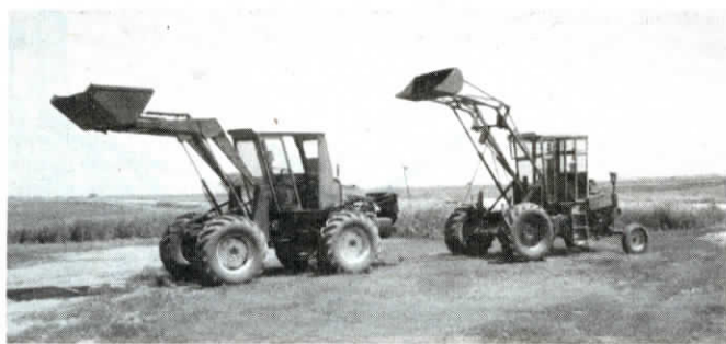
Priefert built both of these tractors out of old Case combines.
