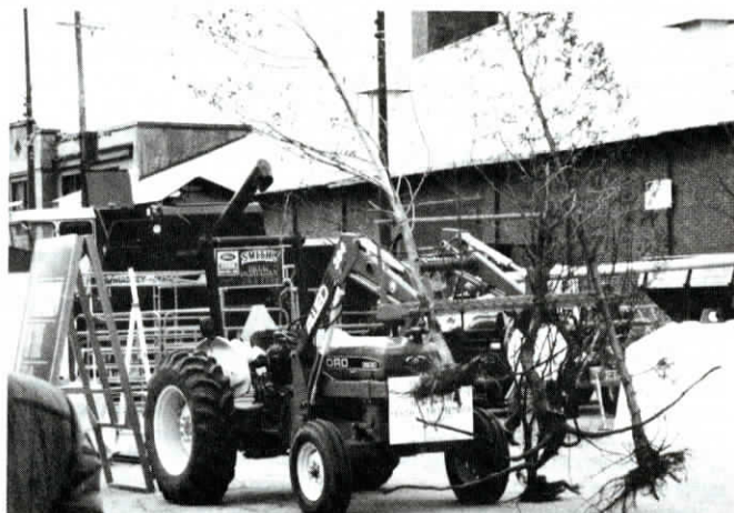
Small trees and brush pass through wide openings at front end of teeth and then get jammed in narrow openings at rear end.
