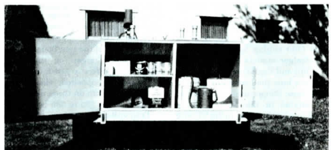
Twin tanks, both ventilated and baffled, hold 235 gal. each. Trailer deck measures 6 by 10 ft. Accessory box in rear has 36.1 cu. ft. of space for oil and grease drums and other parts and accessories.
