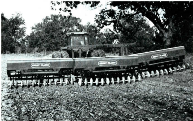
Drill's three 10 ft. sections float independently on uneven ground. It lifts for folding or unfolding.
