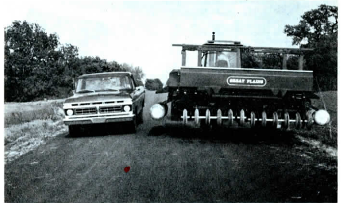
Driver folds the drill hydraulically to narrow 15½ ft. width for road transport.
