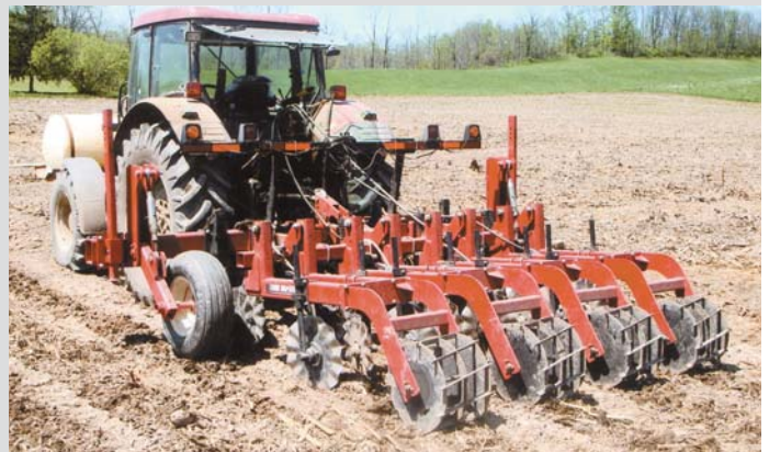
"One time over the field takes the place of plowing, field finishing, and applying nitrogen," says George Mills about his Brillion STP-430 Strip-Till machine.
