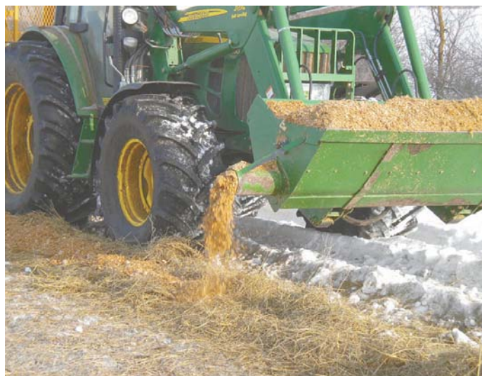
To turn his loader into a mini feeder, Cody Shay installed a hydraulic-powered, 6-in. dia. poly auger in the bucket. An agitator above auger prevents bridging.
