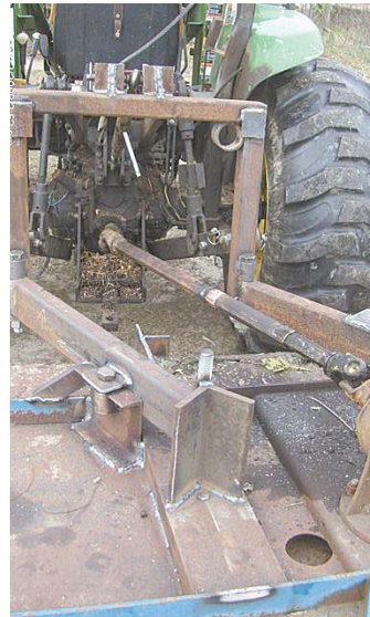
Mower was originally 3-pt. mounted. Greene cut the 3-pt. bracket off the mower and then made an upside-down, U-shaped frame that pins onto tractor's 3-pt. hitch.
