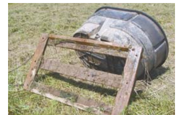
Sled is made from 2 by 6's, with a short length of chain at one end that hooks up to the ATV.
