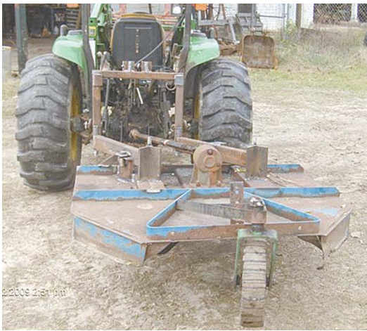
By pulling a pin on an offset hitch, Hobby Greene can shift his tractor mower 16 in. to the side.
