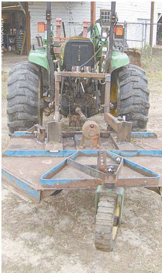
Mower was originally 3-pt. mounted. Greene cut the 3-pt. bracket off the mower and then made an upside-down, U-shaped frame that pins onto tractor's 3-pt. hitch.
