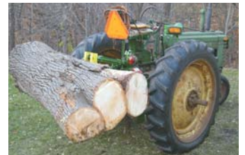
A log lifting attachment for the drawbar can pick up tree trunks of up to 1,500 lbs. with no problem.
