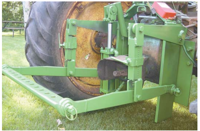
"The drawbar can be lowered to ground level or raised 3 ft. high, which makes it easy to drag logs and to lift heavy trailer tongues," says Bipes.
