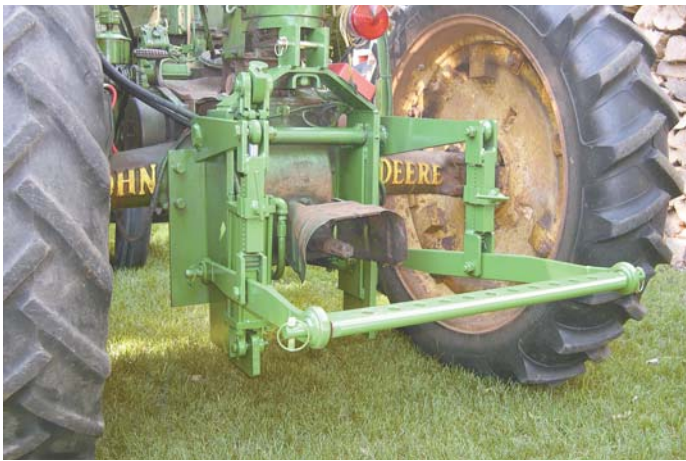
John Bipes replaced the drawbar on his 1940 Deere B tractor with a home-built, hydraulically adjustable, 3-pt. mounted hitch and drawbar.
