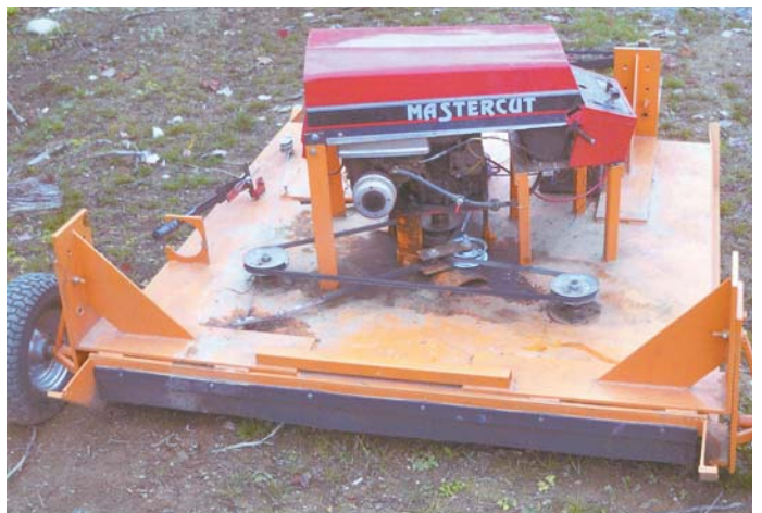
Brian and John Ricker rebuilt their Mastercut riding mower into a low-cost, pull-behind mower to cut their 8-acre lawn. Riding mower's engine, hood and dash mount on top of a home-built, 60-in. deck.
