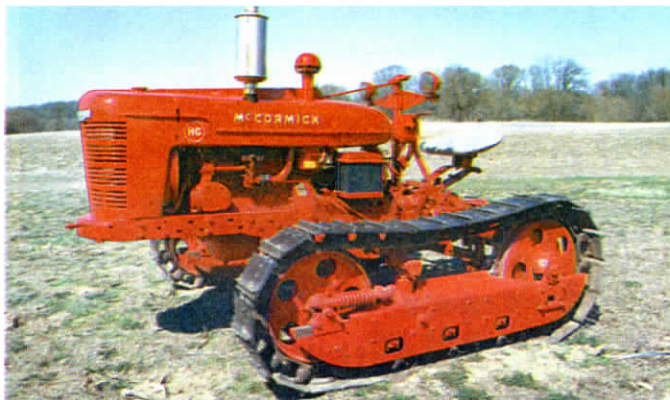
Roller's unique "HC" tractor uses the Oliver's 10-ft. steel tracks, steering brake levers, and rear end. However, it still has the Farmall throttle and clutch pedal.
