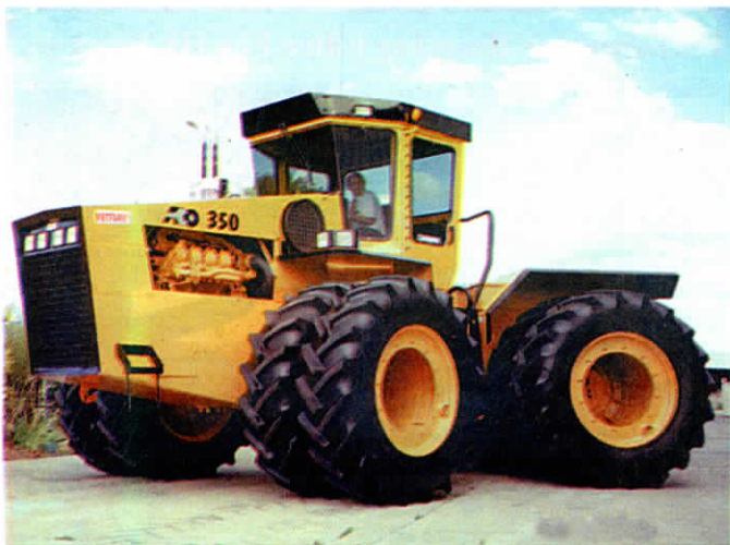
New ACO 490 hp tractor will pull a 39-ft. wide disk plow, using just under 2 1/2 gal. of fuel per acre, according to the manufacturer.
