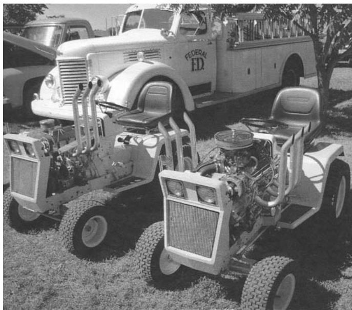
Newly repowered Cub Cadet, right, is equipped with three home-built exhaust pipes on each side.
