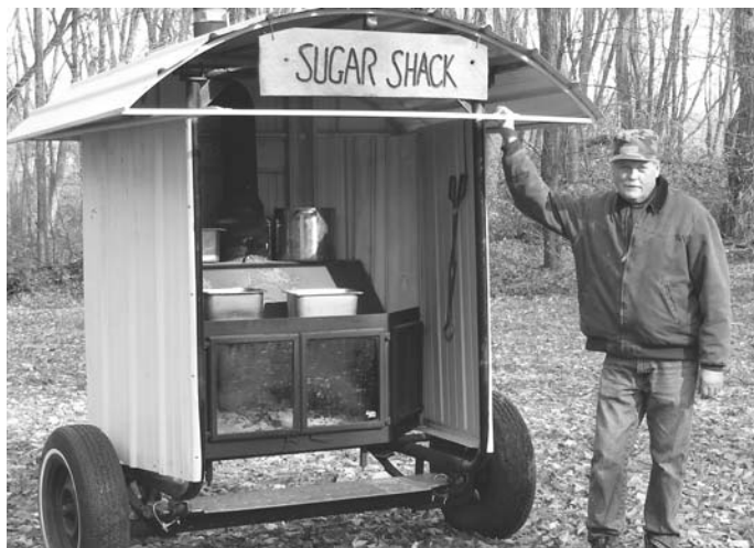
"I made it portable so I could easily put it away in the off-season," says John Siefker about his wood-fired maple syrup cooker.
