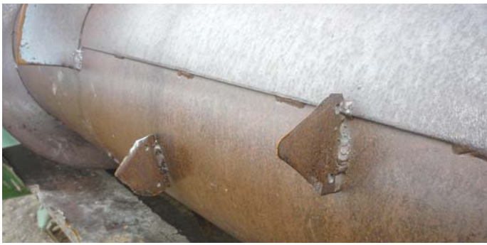
Sickle blade-style grain grabbers are welded into center of auger where they help feed crop material into feederhouse.
