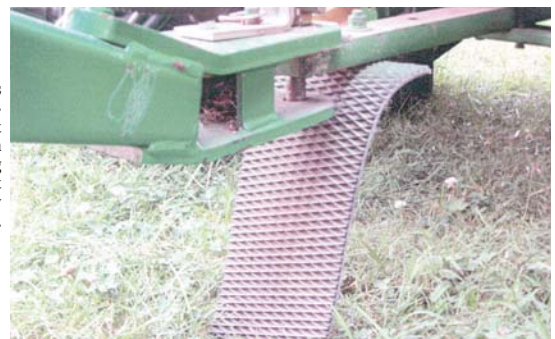
Baler belt hangs freely from tractor drawbar just ahead of hitch pin, compressing windrow so it feeds smoothly into baler.
