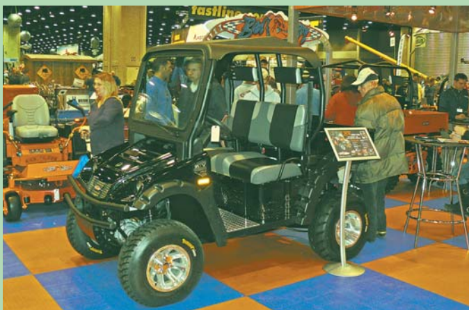
"Bad Boy" electric multi-terrain vehicle runs on eight 6-volt batteries and is recharged by plugging into a standard wall socket.
