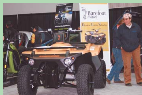
Electric-powered ATV is powered by lithium iron phosphate batteries. They're said to last up to four times longer than ordinary lead acid batteries.
