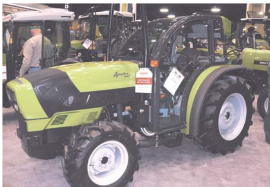
Deutz-Fahr F320 tractor is fitted with a special order cab with great visibility. Glass extends from the hood to well past the driver's head.
