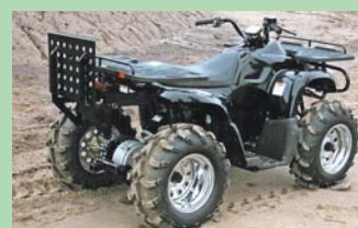
E-Force ATV is powered by a 72-volt, brushed DC motor with up to 28 hp.
