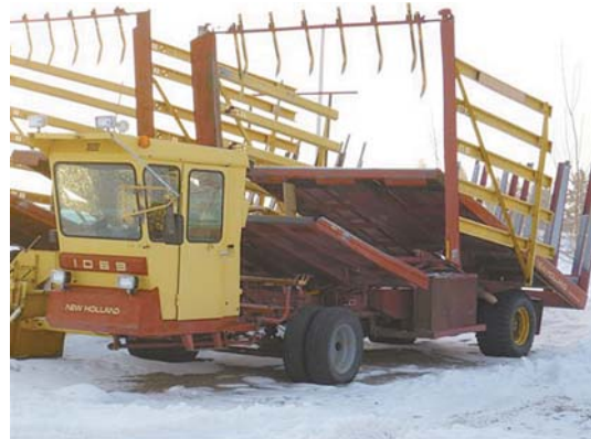
Peter Fehr put a bigger engine in his New Holland Bale Wagon and also stretched the table and frame 18 in. to hold more bales.
