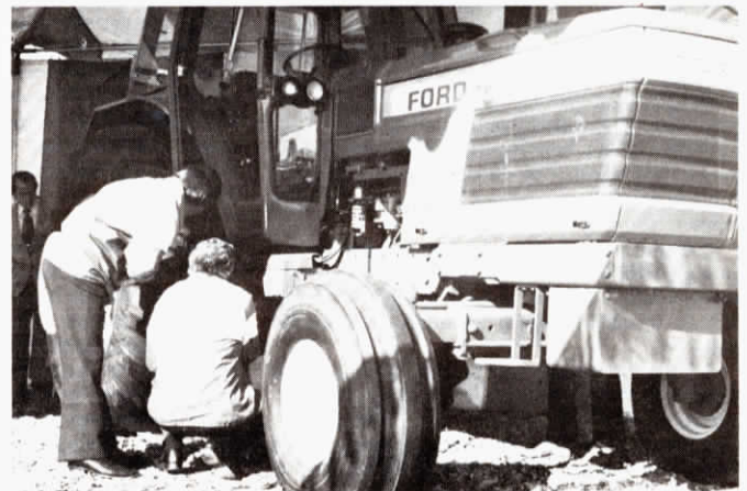
Top of the line for Ford's two-wheel drive tractors is the TW-30, powered by a new turbocharged, intercooled Ford diesel engine with 163 pto horsepower.
