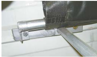
Four pieces of 3/4-in. metal conduit, each bent to an L-shape, hold tarp over machine.
