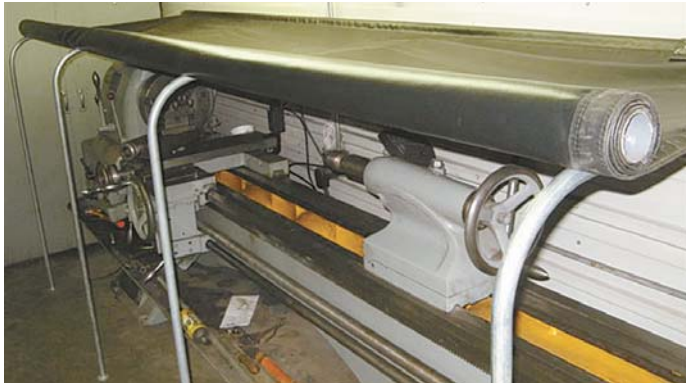
Tarp keeps dust and dirt from collecting on Roger Gutschmidt's metal turning lathe.
