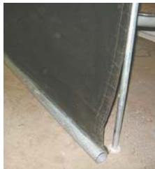
Four pieces of 3/4-in. metal conduit, each bent to an L-shape, hold tarp over machine.
