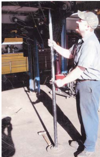
"Third hand" consists of a larger pipe welded to a brake rotor base, and a smaller telescoping pipe welded to a U-shaped plate that supports the work.
