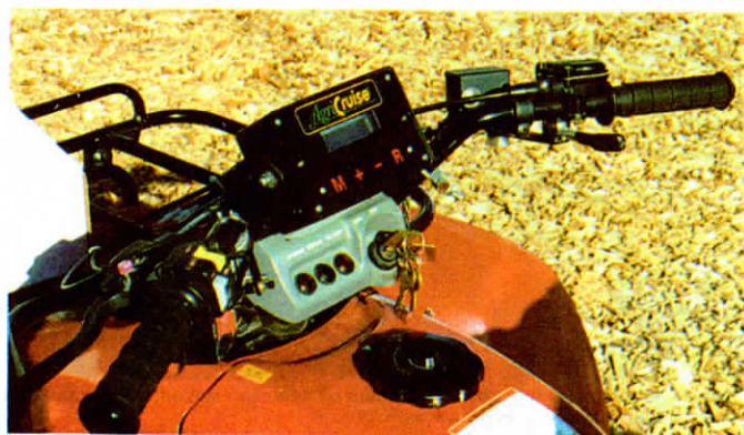
Electronic monitor mounts on handlebars. Throttle control unit on front rack.
