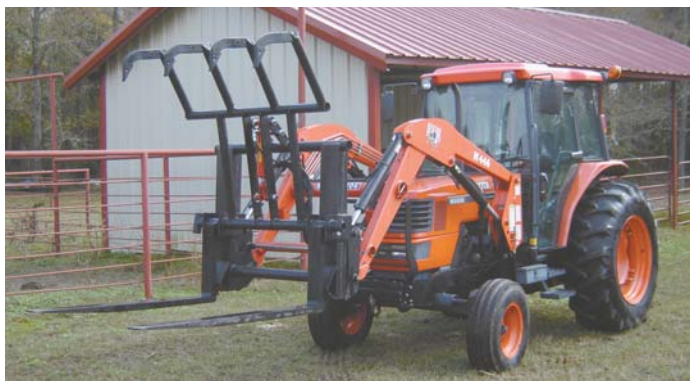
After years of ice storms, tonados and draught, Calvert finds plenty of use for his home-built brush grapple.
