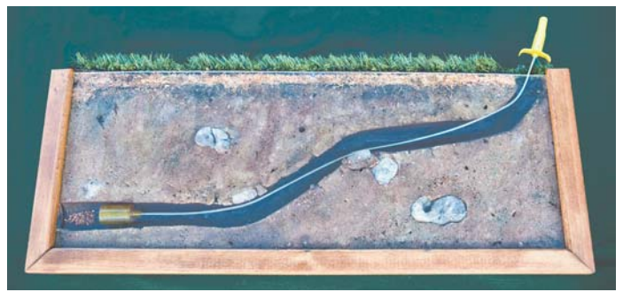
Gopher bait applicator deposits bait deep in gopher tunnel. It's made from a 28-in. flexible metal cable and a 1 1/4-in. dia. clear plastic bait chamber with a spring-loaded control handle.
