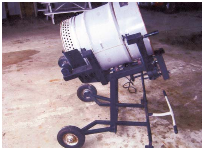
Dirt falls through holes drilled into sides and bottom of rotating drum.
