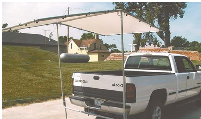
Tailgate canopy has a fabric top that attaches to a frame made from round tubing. It provides shade over a 7 by 12-ft. area.
