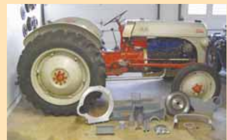
Photo shows parts included in overhead valve conversion kit for N-Series Fords.
