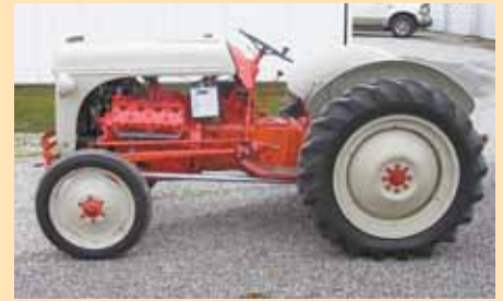
Kit costs $1095 and contains all the hardware needed to connect the V-8 engine and clutch assembly to the Ford 8N transmission and frame. Knasel says it takes about 8 to 10 hours to install.
