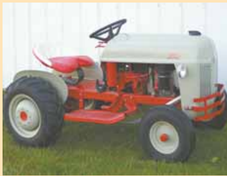
Single piece fiberglass hood fits over most standard garden tractors.
