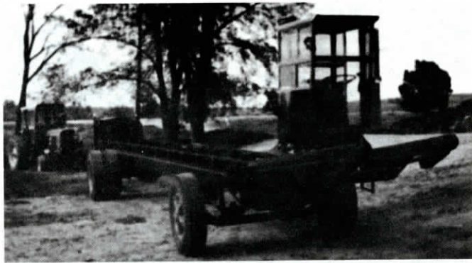
Up-front ramp lowers to ground to pick up bales, and raises to load bales up onto trucks, if necessary.
