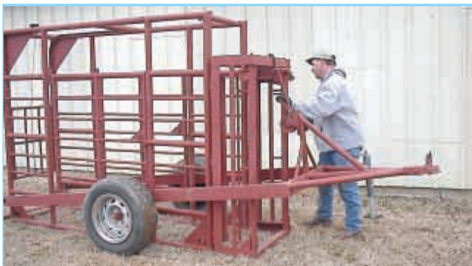
Michael Haynes used salvaged 1 1/4-in. pipe and other material to make this portable cattle chute.
