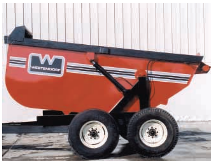
Westendorf Mfg.'s new Dump Spreader gradually raises on-the-go until it reaches a 90 degree tilt that allows all the material to be unloaded.
