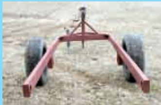
Trailer that carries chute has a horseshoe-shaped frame made from 4-in. channel iron.
