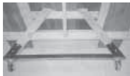
He bolted channel iron to legs and then welded coaster wheels to the channel iron.
