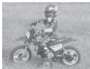
Training wheels bolt on under middle part of motorcycle, allowing rider to lean into them without falling over.
