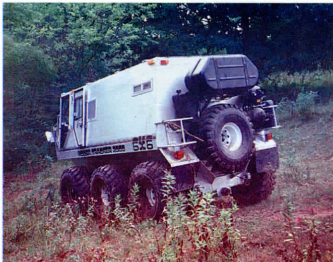
Moose Tracker 6-WD was built over a period of two years from combine parts.
