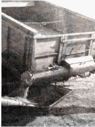
Unit's 9 in. auger unloads to the side of the truck, or through center endgate.
