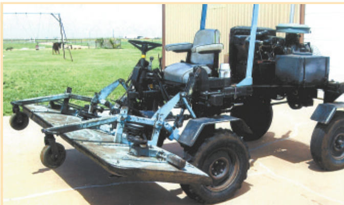
Daryl Dixon converted an old Schweiss self-propelled bean buggy into this 8-ft. articulated riding mower. The rig's pto-driven deck is home-built.
