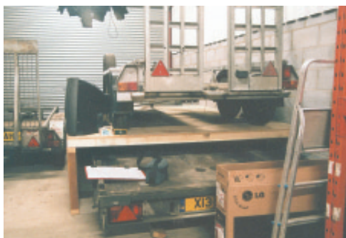
Tony Hudson can store two flatbed trailers in the space of one. Ramps run up to top level to park a second trailer on top.
