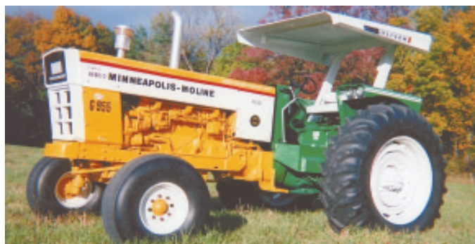
Irvin Seibel's unusual G-955 tractor has a Minneapolis Moline front end and an 1855 Oliver rear end.
