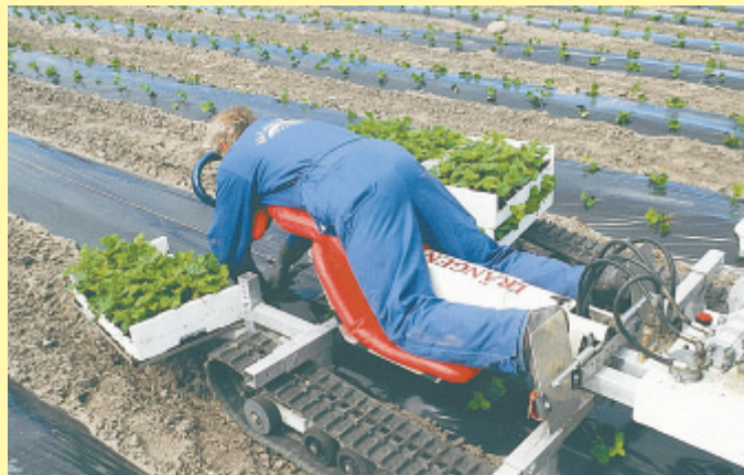
Drangen work cart makes it easier to work vegetable and berry patches. The operator steers and controls speed of cart with his feet.
