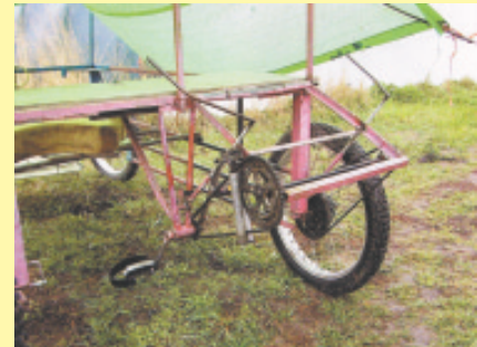
Robert Hettler built this "straddle buggy" to take some of the pain and drudgery out of planting and weeding. Overhead tarp provides sun and rain protection.
