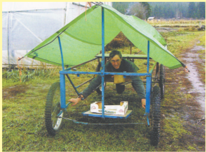
Robert Hettler built this "straddle buggy" to take some of the pain and drudgery out of planting and weeding. Overhead tarp provides sun and rain protection.
