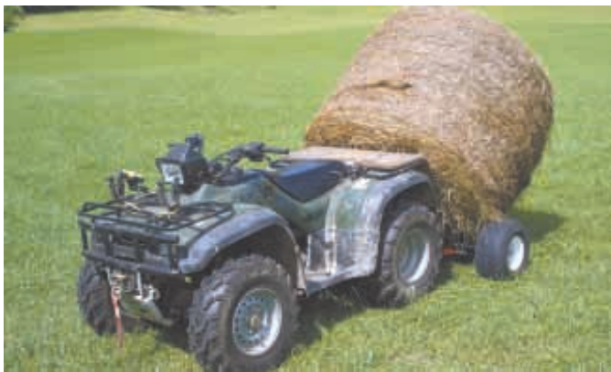
Hay Baby uses an electric-operated winch to raise or lower speared bales.
