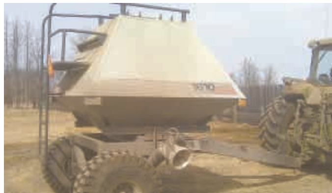
Howard Goertz and his sons converted a Flexi-Coil air seeder into a pellet-feeding wagon.
