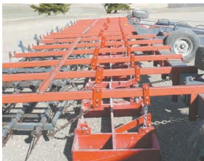
“Mole Hill Destroyer” is an add-on device for land drags that’s designed to make mole hills and gopher mounds disappear.
