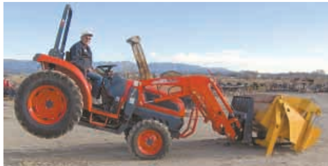
Before the front axle was moved forward to lengthen the wheelbase, this tractor had trouble lifting the load.
