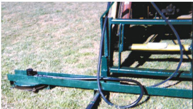
Mower is powered by tractor's hydraulic system.
