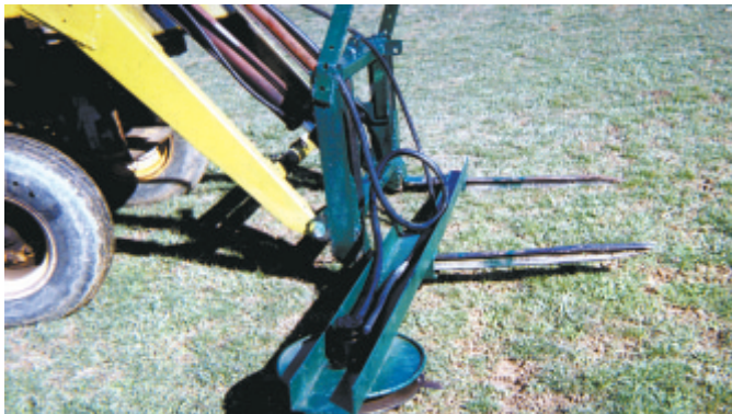
Mower attaches to loader-mounted forks. It consists of four disc mower blades attached to a metal skid plate. Blades cut a 2-ft. wide strip under fences.
