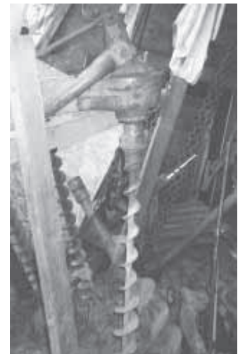
Gilbert Conn uses a 4-in. dia. auger to drill pilot holes for fence posts. Post can then be pushed in tight with a loader with no need for tamping.
