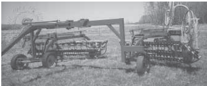
Home-built hitch lets Gleason trail his left and right hand basket rakes down the road.
