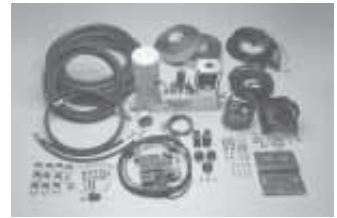
Flex fuel kit is tied into vehicle's ignition system. It allows you to flip back to diesel from an alternative fuel by simply flipping a switch.
