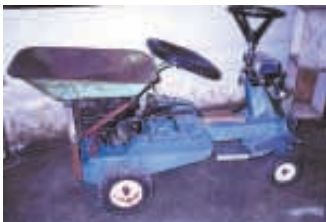
Self-propelled wheelbarrow was built out of a late 1960's Ford riding mower.
