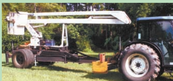
Wayne Beauchamp's cherry picker began life on an electric power company truck. He mounted it on wheels and powers it with the tractor's hydraulic system.
