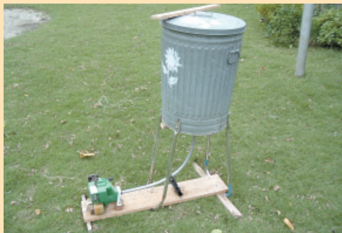
Billy Robb's mini threshing machine consists of a trashcan and a weed trimmer. It shreds leaves, stalks and seed heads in minutes. Seeds fall out the bottom of the can.
