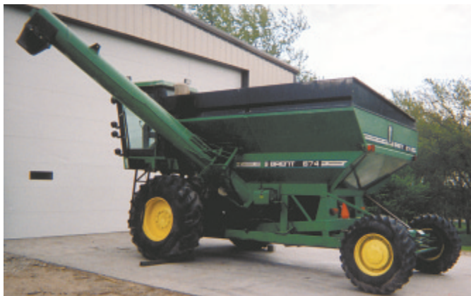
To make this self-propelled grain hauler Harlan Schlaak combined a Deere 8820 combine with a 674 Brent grain cart.
