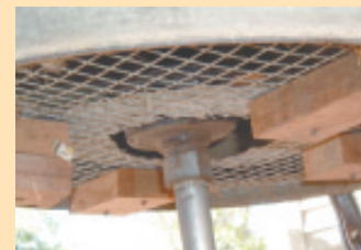
Billy Robb's mini threshing machine consists of a trashcan and a weed trimmer. It shreds leaves, stalks and seed heads in minutes. Seeds fall out the bottom of the can.
