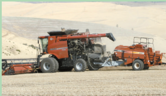
Case 8010H combine pulls Hesston 4790 baler, harvesting grain and straw at same time. All residue from combine is funneled directly into the baler.
