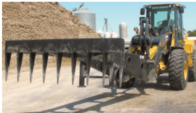
Heavy-duty silage rake is available in 12- or 16-ft. wide versions that mount on front of an industrial loader tractor. The 2-ft. long spear-like teeth are spaced 14 in. apart.
