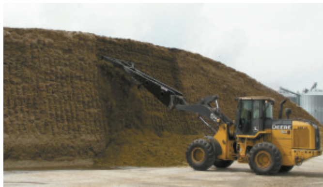
Operator rakes silage from stack and then quickly switches to a bucket or grapple fork for loading.
