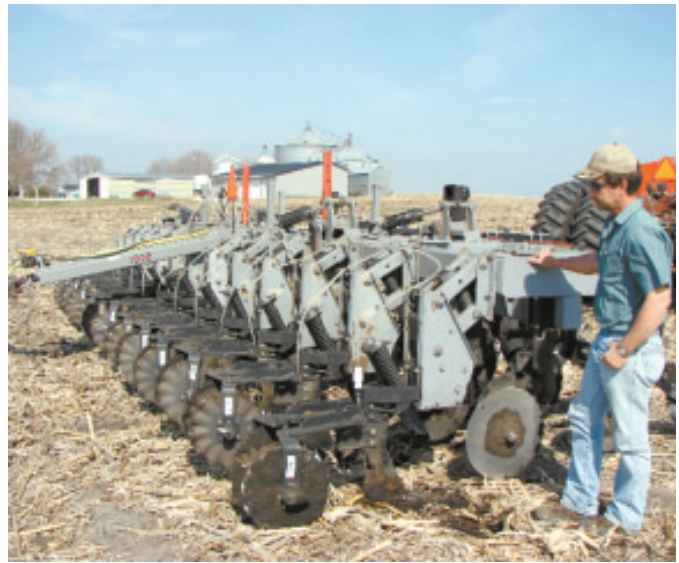
Tim Renger and his father, Bucky, built this 13-row strip-till rig and fertilizer applicator from used cultivator toolbars.
