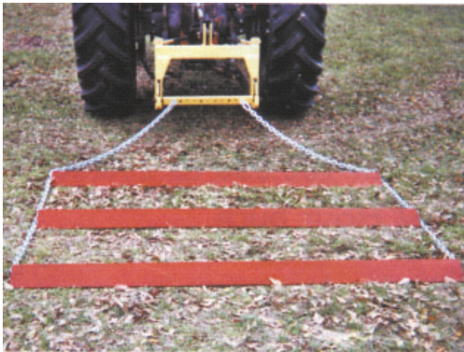
Heavy-duty implement breaks up manure piles and spreads the material over pasture.
