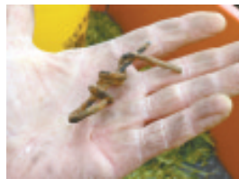
This small piece of rusted fence wire was found in the machine.
